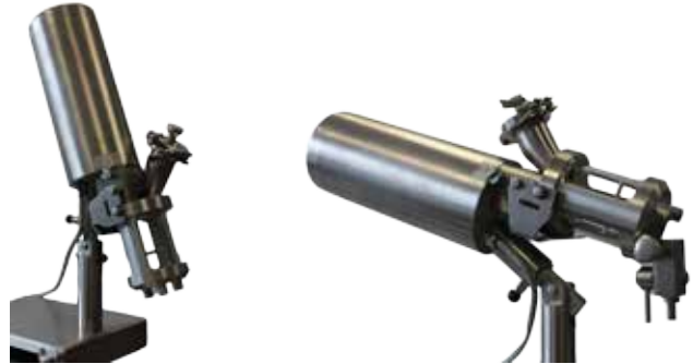
Micro metering screw PMD, shown in the two different setting angles
