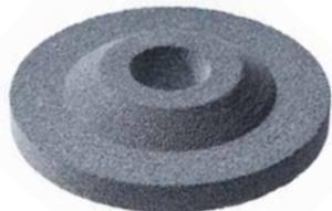
The Corundum Disk Mills are used for wet milling and homogenizing of liquid, viscous and pasty products. The corundum disks are available in different grain sizes acc. to the required fineness. The axially movable stator is pressed against the rotor which is running at high speed. Due to the high shear forces
