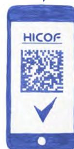
For authentication Hicof works with off the shelf smartphones including even those from the last generation. In order to check suspect products simply the Hicof App needs to be installed. The App is available for the most common operating systems and is optimized to scan codes in dark environments without the need for special lenses or special lamps.
