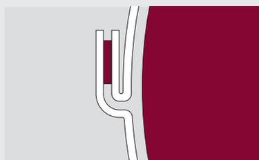
Sealing & folding the seam
